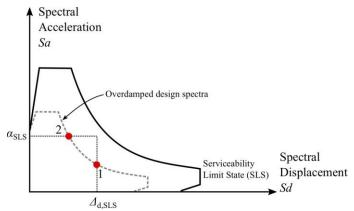
Figure 16. Example of when SLS performance objectives cannot be met and some solution in the form of base isolation or supplemental damping is required.
