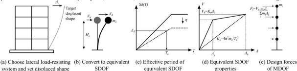
Figure 8. This gave a simple and direct method of seismic design which culminated in the development of direct displacementbased design (DDBD) described in Priestley *et al.* [19]. This was proposed as a suitable alternative to FBD as it possesses advantages in terms of design approach and it is arguably better aligned for the objectives of PBEE, whereby performance levels can be linked to levels of structural demand rather than forces.
