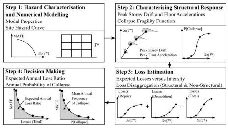
Figure 1. Overview of the PEER PBEE framework used to estimate the EAL and MAFC of an existing building (adapted from O'Reilly et al. [11]). Note: MAFE denotes mean annual frequency of exceedance, whereas Sa(T\*) refers to the spectral acceleration at a period T\*.
