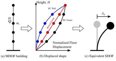
*Figure 12. Identification of*  $\Delta_d$  *for different structural systems.*
