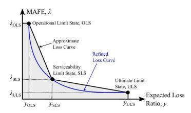
Figure 9. Illustration of approximate and refined loss curves, where integrating the expected loss ratio, y, with MAFE,  $\lambda$ , gives the design EAL. Note: the vertical axis is plotted using a logarithmic scale for illustration purposes.
