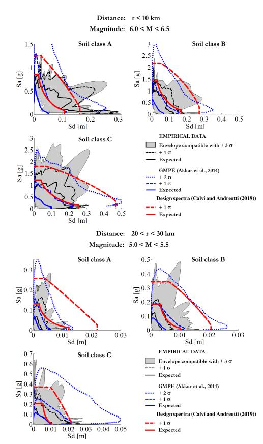
Figure 4. Comparison between design spectra proposed by Calvi and Andreotti [3], derived from the GMPE by Akkar et al. [16] and response spectra empirically derived from signal analysis.
