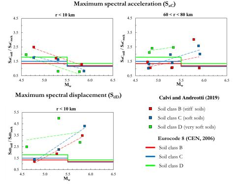
Figure 3. Variation of soil amplification factors with magnitude, distance and type of soil and comparison with S factor of Eurocode 8 (from Calvi and Andreotti [3]).
