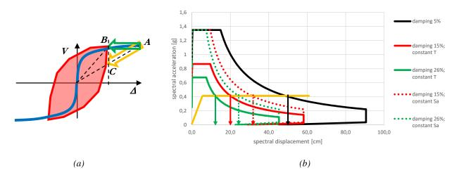
Figure 6. Capacity spectrum assessment of a structure with assumed shear strength equal to 40 % of its effective weight, for different equivalent damping and correction of the displacement spectrum
