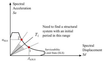
Figure 13. Identification of permissible initial secant to yield period range based on PFA and PSD limits for the SLS.
