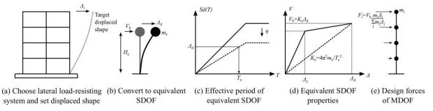
Figure 8. Basic steps of DDBD [19]: (a) lateral load-resisting system is chosen and target lateral displacement profile set (b) equivalent SDOF system identified, (c) effective period,  $T_e$ , is identified, (d) design base shear,  $V_b$ , is identified and (e) lateral forces, F, distributed.
